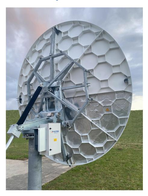
HILTRON Communications has introduced a field-upgradable motorisation kit specifically designed for existing fixed installations of CPI 2385 Series 3.8 metre Rx/Tx antennas in current deployment for tracking applications, or for new installations requiring tracking functionality.
