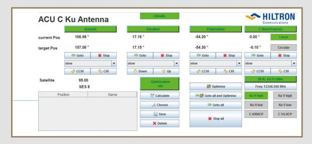
Besides position, drive and tracking control the GUI allows control-access to linear/circular switch, beacon receiver, signal matrix and cabinet temperature conditioning.
