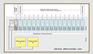
Hiltron Control System - HCS: Schematic Diagram of System implemented in 19"/2U chassis with 16 modules capability
