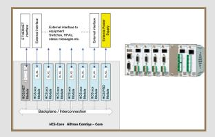
Hiltron Control System - HCS: Schematic Diagram of System implemented in chassis with 8 and 16 modules capability
